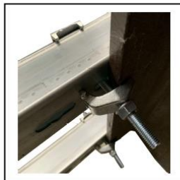
Tighten the 8 nuts
